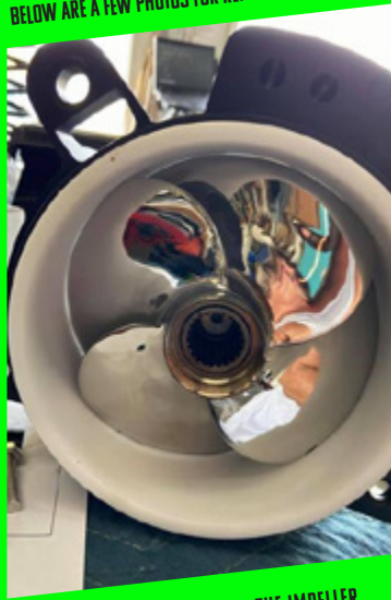
NOTICE THE CLOSE GAP BETWEEN THE IMPELLER AND THE WEAR RING. THIS IS NORMAL.
