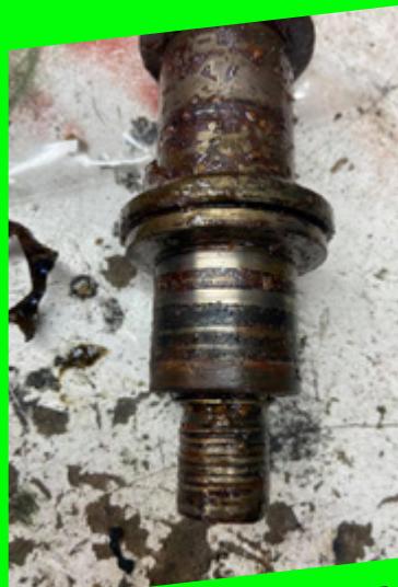
THE IMPELLER SHAFT FROM THE JET PUMP THAT LET WATER SEEP IN AND DESTROY THE BEARINGS.
