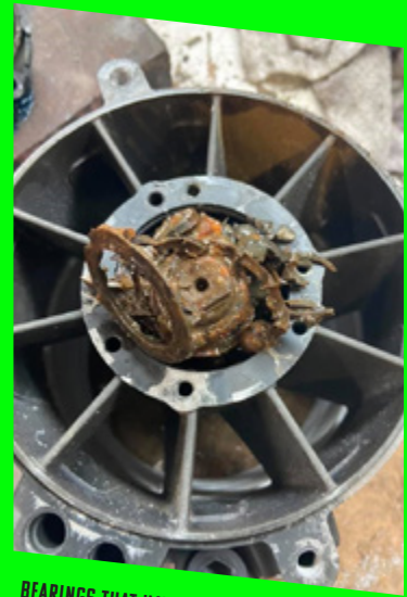
BEARINGS THAT HAVE WATER INSIDE THE HOUSING. THE BEARINGS RUSTED OUT AND BLEW APART.
