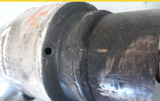
EXAMPLES WHERE WATER BLEEDS INTO THE EXHAUST STREAM BEFORE ENTERING THE WATERBOX
