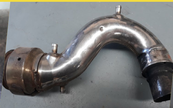
EXAMPLES WHERE WATER BLEEDS INTO THE EXHAUST STREAM BEFORE ENTERING THE WATERBOX
