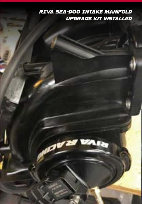
RIVA SEA-DOO INTAKE MANIFOLD UPGRADE KIT COMPONENTS.
