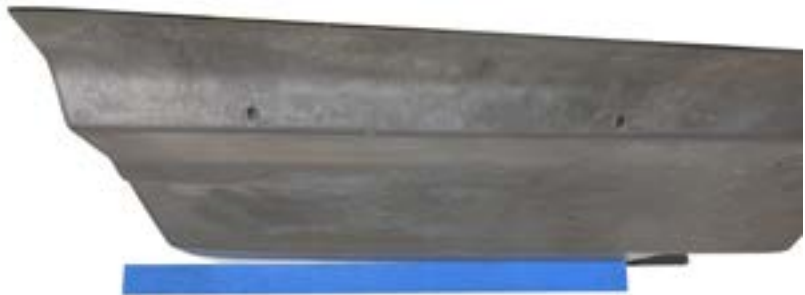
Planing surface angle change begins 6" after intake grate mount
