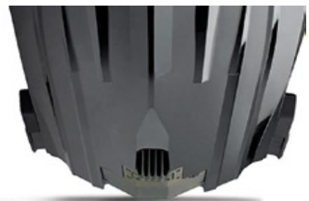
VIEW OF UNDERSIDE OF PERSONAL WATERCRAFT AT JET PUMP INLET (STOCK INTAKE GRATE)
