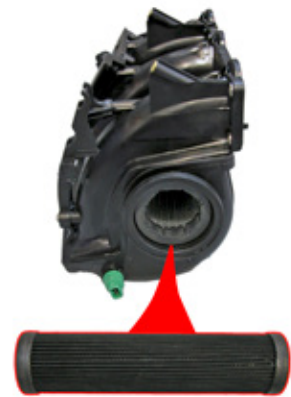
RESTRICTIVE MESH ELEMENT REDUCES AIR FLOW INTO ENGINE ROBBING IT OF HORSEPOWER.
