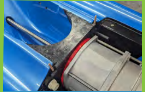
Custom CF Pump Shoe & installation tool
