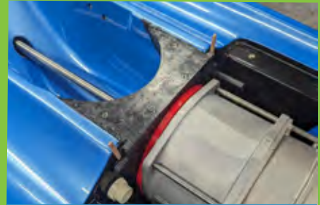
Custom CF Pump Shoe & installation tool
